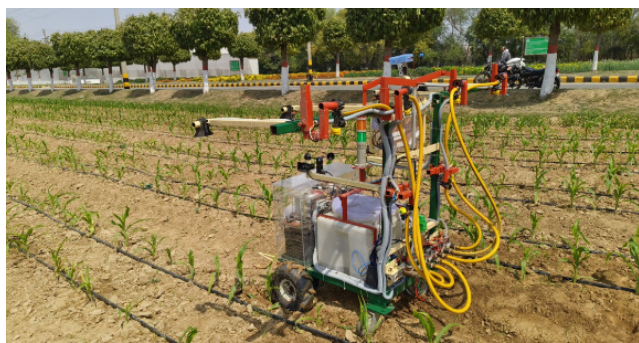
Telerobotic Target-Specific Pesticide Applicator
