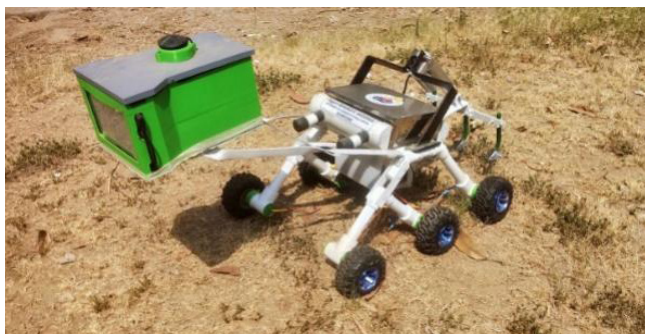
Weed Detection and Light Tillage Robot
